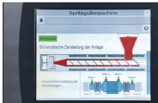
The online system's panel on the CM box; the data from the individual sensors can be viewed here
